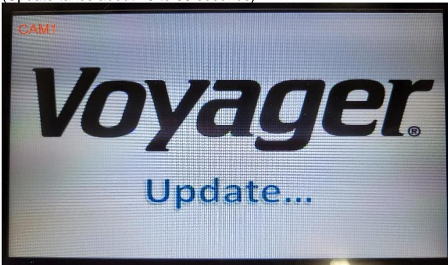
4. Once Updating is completed it will say 'Update Successful,' at this point remove and cycle the Power on the Module.
